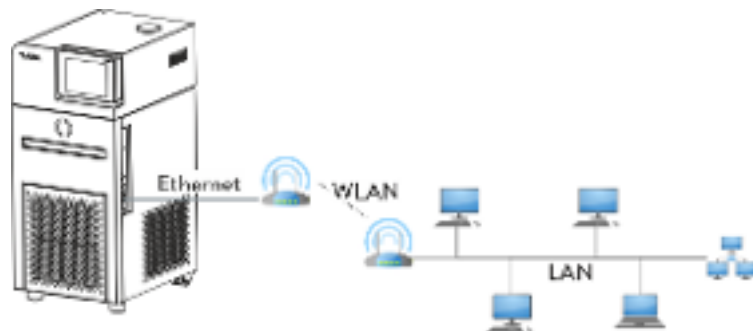
Fig. 16: Connected via LAN and WLAN
