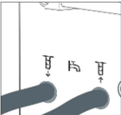
Fig. 23: Cooling water input and output
