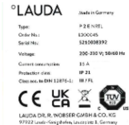
Fig. 12: Rating label for a heating thermostat (example)
