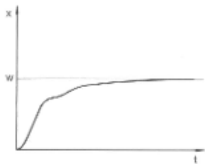
Fig. 53: Control parameters T_n and T_v too large
