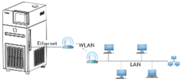
Fig. 16: Connected via LAN and WLAN
